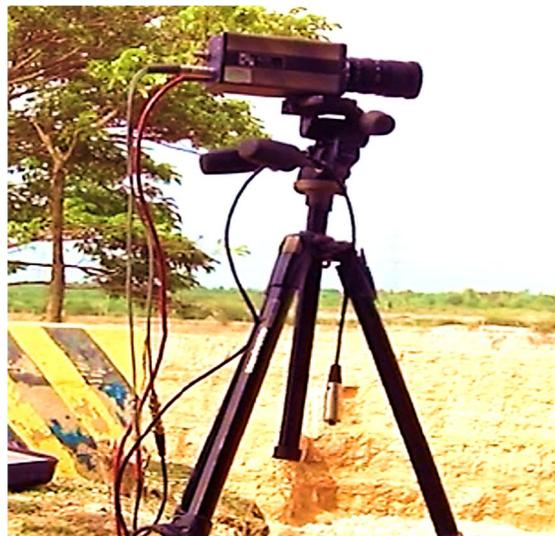
Figure 2. High speed video camera of 1000fps capacity
