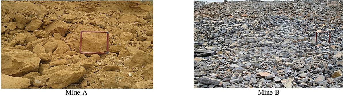
Figure 5. Typical muck pile obtained from the blasts
